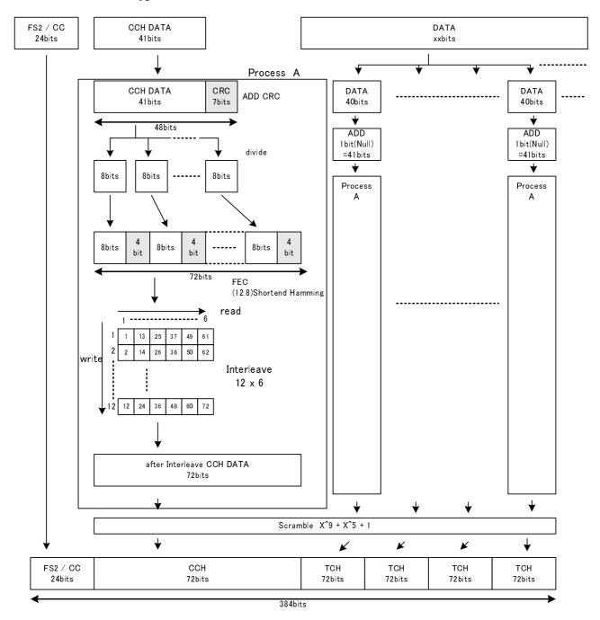
Figure 8: Type 2 data frame coding
