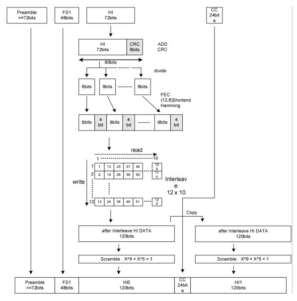
NOTE: Header Frame Channel Coding.
