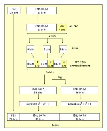
Figure 11: End frame coding
