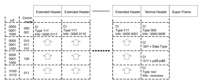
Figure 12a: Extended header coding
